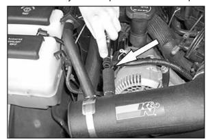
20. Re-connect the crankcase vent hose to the  $K\&N^{\otimes}$  intake tube as shown.
