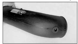
18a. After marking the intake tube, remove the tube from the vehicle and drill a 5/8" hole into the intake tube then install the provided grommet as shown.
