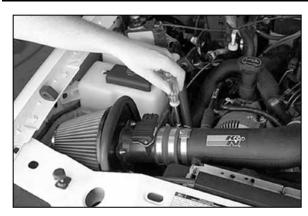
23. Install the heat shield assembly onto the K&N® intake tube and tighten the hose clamp as shown.
